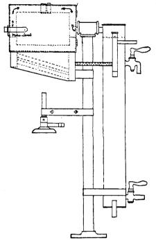
the result of the heat applied to their outer surface. The source of heat is an ordinary Bunsen burner, used with a wing-tip, so as to spread the flame over the surface of the pipes. The pipes are of small diameter so as to afford a large heating surface in proportion to the amount of water passing through them.
